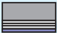
EC-110 - Semi-closed EPDM foam - Acrylic based adhesive - Non woven carrier - Acrylic based adhesive - Release liner
