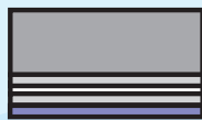
EC-130 - Semi-closed EPDM foam - Acrylic based adhesive - Polyester carrier (12 µm) - Acrylic based adhesive - Release liner
