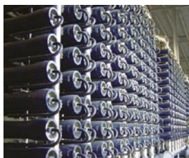
Reverse osmosis membrane modules for seawater desalination system
