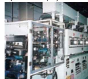
■ Solvent-free adhesive tape prototype fabrication machine
