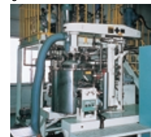
■ Solvent-free adhesive tape prototype fabrication machine
