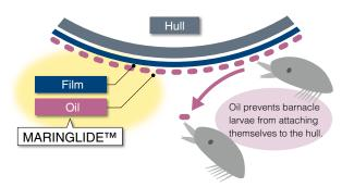
A very small amount of oil is released from the surface of the film to prevent biofouling.
