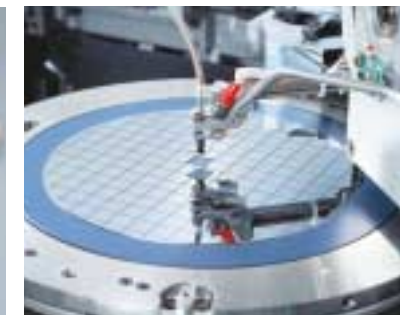
Wafer pick-up system The system is used in the wafer back-grinding process and dicing processes that are part of semiconductor manufacture.
