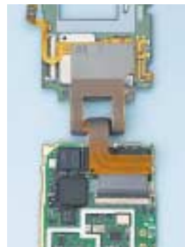
High flex fatigue life flexible printed circuit This highly reliable flexible circuit board was developed for applications that require repeated bending.
