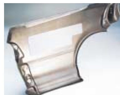
Reinforcing and vibration damping material (NITOHARD®) This epoxy resin foam sheet is affixed to the steel plate lining of automobile bodies to not only improve rigidity but also to attenuate vibrations, noise and heat.
