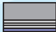
EE-1040 - Semi-closed EPDM foam (EE-1000) - Butyl-based adhesive - Cloth carrier - Butyl-based adhesive - Release liner
