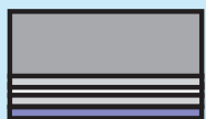
EE-1010P - Semi-closed EPDM foam (EE-1000) - Acrylic-based adhesive - Polyester carrier - Acrylic-based adhesive - Release liner
