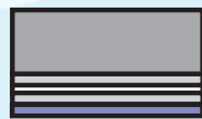
EE-1010 - Semi-closed EPDM foam (EE-1000) - Acrylic-based adhesive - Non-woven carrier - Acrylic-based adhesive - Release liner
