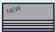
EE-1010EP - Semi-closed EPDM foam (EE-1000) - Acrylic-based adhesive - Non-woven carrier - Acrylic-based adhesive - Release liner
