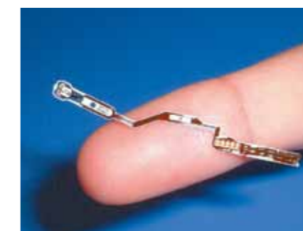
"CISFLEX®", our thin-film metal base board with high resolution circuit
