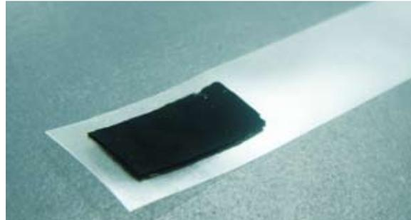
Gecko tape; black area is 'hair' made of carbon nanotubes.
