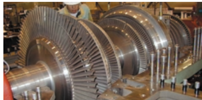
Steam turbine that produces electricity
