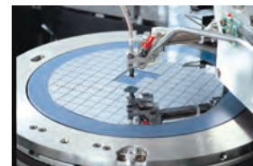
Dicing tape that enables damage-free pickup of thin-film chips
