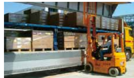
Example of application of "Cargo Deck" (The blue shelf is the "Cargo Deck")
