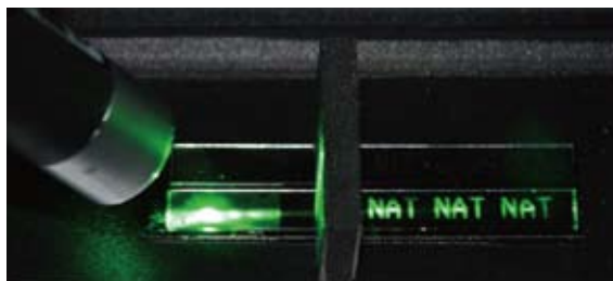
An optical waveguide Light, which enters from the left hand side, passes through the waveguide. The waveguide is a light path formed by precision polymer processing and is located at the bottom of the center wall. The letters, formed by the waveguide, appear on the right hand side.
