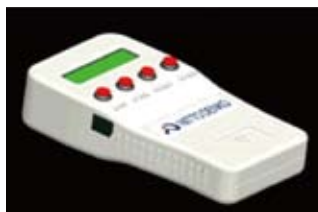
A typical optoelectronic sensor The biometric information can be obtained instantly by inserting a sample into a small portable device.
